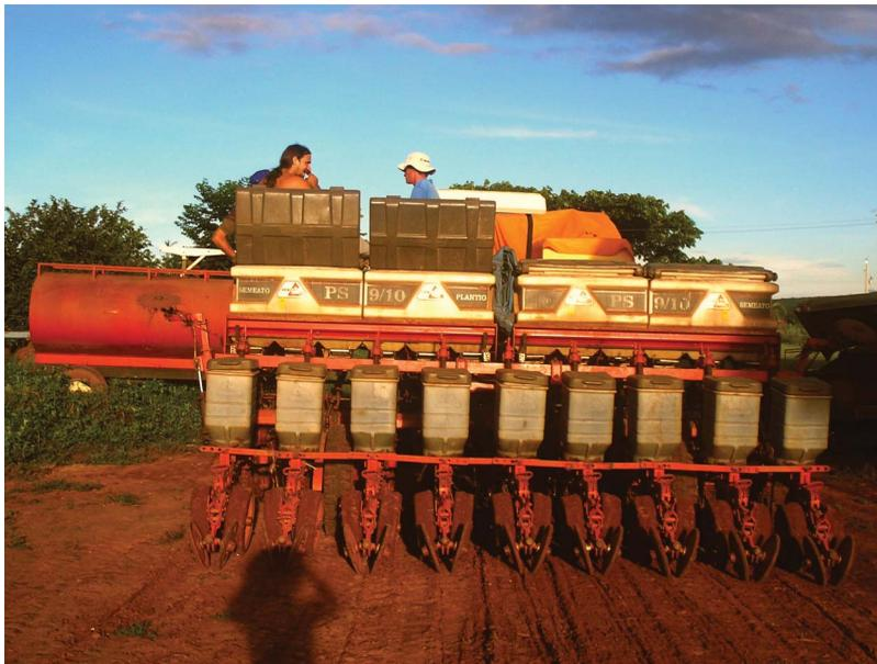
**FIGURE 6** Planter machine used for direct-seeding in-rows, Mato Grosso State, west-central Brazil (Credit: Luciano Langmantel Eichholz) (color figure available online).
