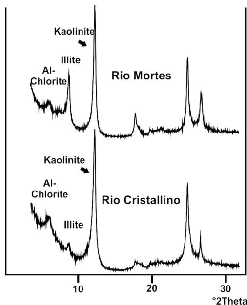
**Fig. 6** X-ray diffraction of  $<2\text{-}\mu\text{m}</math> samples of suspended matter from the Das Mortes and Cristalino Rivers, both of which drain the Araguaia plain, either mostly or exclusively$
