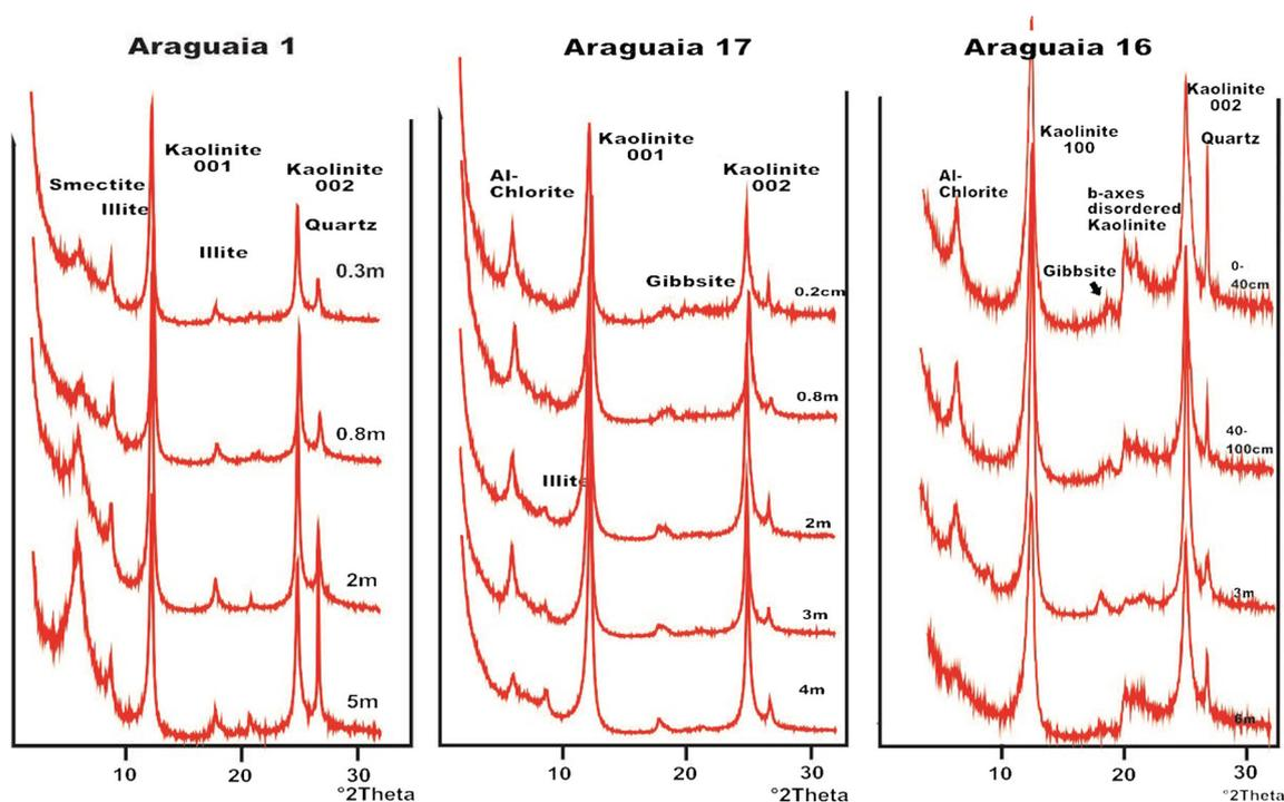
**Fig. 4** X-ray diffraction of  $<2\text{-}\mu\text{m}$  samples from a 5-m sediment profile of the sub-recent sediments of the Araguaia River near Cocalinho city (Araguaia 1, left), a 4-m profile in the active paleo-floodplain south of São
